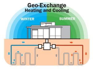
The geo-exchange bores are used in our climate, with cold winters and hot summers, to exchange heat and maximize energy-efficiency year round. The geo-exchange system uses a heat pump to store and retrieve heat from the earth, often called a *ground-source heat pump*. A conventional furnace burns a fossil fuel to produce heat, a geo-exchange system **transfers heat** from one place to another.
